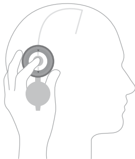
Fig. 9: Localising the valve using the M.blue Compass
